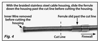
Step 7: If the Throttle Cable has the braided stainless steel housing, wrap tape around the cable housing at your mark and use a cutoff wheel or fine-toothed hacksaw to cut the cable housing. If the Throttle Cable has the black universal or Vintage Series housing, cut the cable housing at your mark with heavy duty 8" diagonal cutting pliers or a hacksaw. Lokar recommends Klein brand Diagonal Cutting Pliers, # D2000-28 available at The Home Depot or through W. W. Graingers, part # 4A838.
