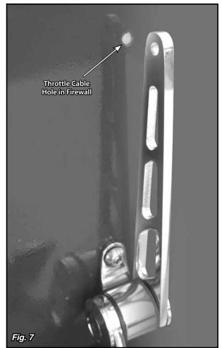
NOTE, Aluminum Pedals Only: Once the Throttle Cable is installed and all adjustments have been made, remove the set screw in the lower arm using a 3/32" Allen wrench.
