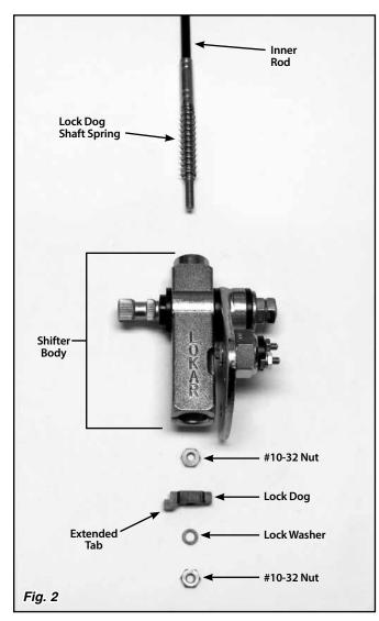
Step 9: Apply a generous coat of synthetic multi-purpose grease to the inner rod. Slide the new Shifter Lever over the inner rod and screw the lever all the way into the shifter body until it stops. DO NOT use thread locking compound on the Shifter Lever. Then, unscrew the Shifter Lever three full turns and line it up straight with the bend towards the rear.
