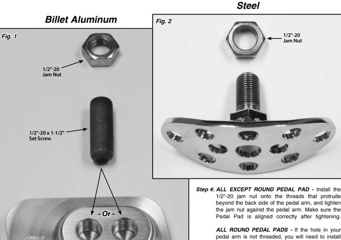
1/2"-20 iam nut onto the threads that protrude beyond the back side of the pedal arm, and tighten the jam nut against the pedal arm. Make sure the Pedal Pad is aligned correctly after tightening.
