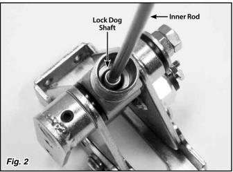
Step 6: If the shifter assembly was removed from the vehicle, reinstall the shifter assembly onto the vehicle. Push down on the inner rod and put the shifter into the "PARK" position, and connect the linkage.
